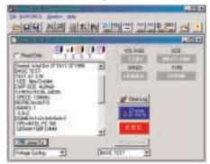
Allows you to print and log test results, with full control of RAMCHECK via the PC. A much more detailed test log and additional measurements are viewable on the PC screen.
