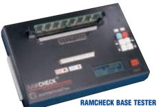
The RAMCHECK base tester comes with a 168-pin test socket and supports all popular PC150/133/100/66 and older ED0/FPM DIMM modules. RAMCHECK is included in the RAMCHECK PLUS package, and can also be purchased separately.
